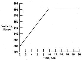
Fig. 5 Variation of velocity for level acceleration from Mach 0.8.
